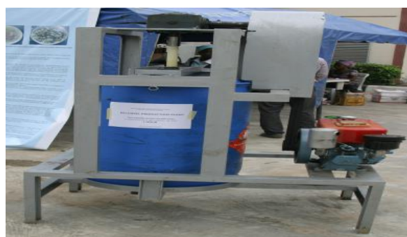
Figure 4: The Hetero-sonic Agitator (HA) with Acoustic Spectral Control (ASC).
